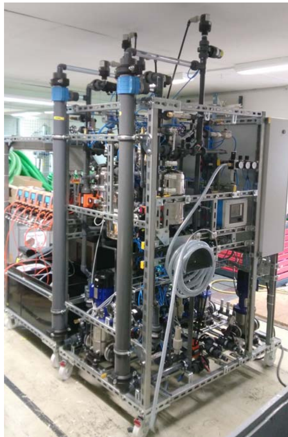
Planned treatment chain for purification of Tai Hu water and ozone depletion after flocculation and membrane filtration (bench scale experiments)
